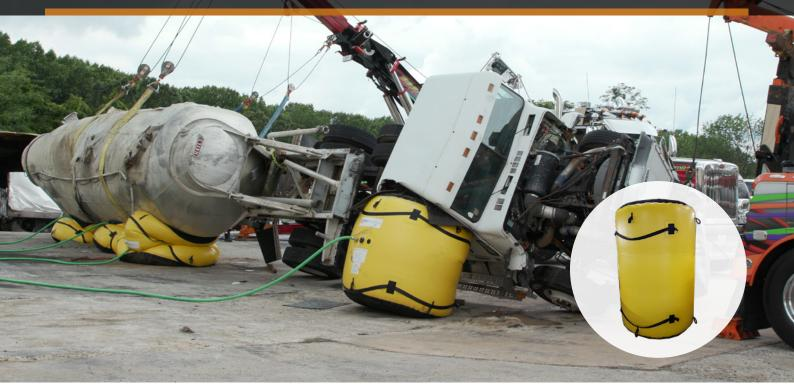
MFC International offer a range of 0.5 bar pressure high lifting bags designed primarily for the recovery of larger, heavier vehicles and trailers.
